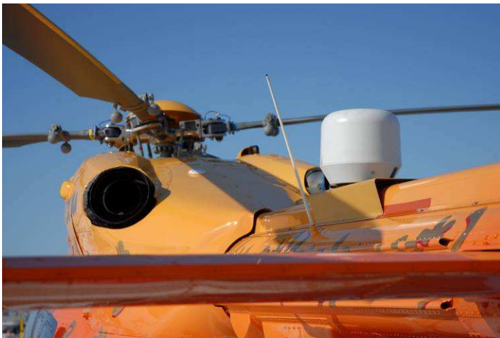
SATCOM antenna on the tail boom
